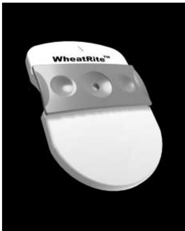
Fig. 8 The WheatRite test cassette for immunoassay of amylase in sprouted grain. An extract of crushed grain is spotted onto the card, which is then closed to permit immunochromatography to take place. The degree of sprout damage is indicated by the intensity of a colored band appearing in the window of the closed card. (View this art in color at www.dekker.com .)
