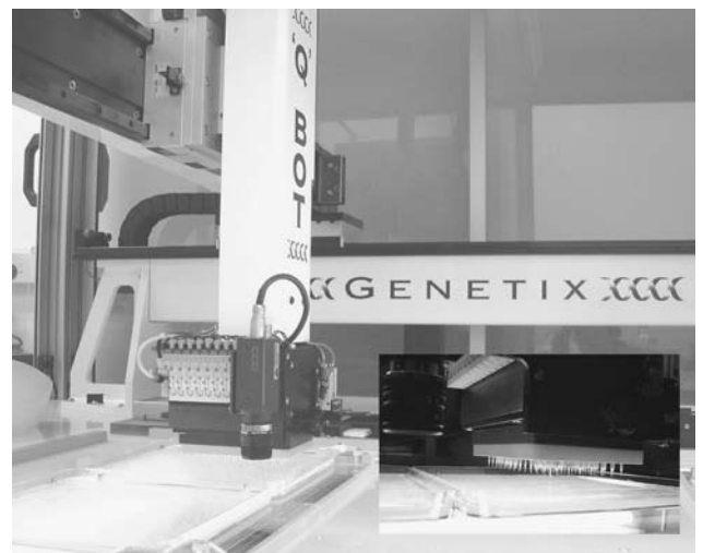
Fig. 1 Laser-equipped robots, such as the “Q-bot” (Genetix LTD, Hampshire UK) shown here, provide fast and accurate handling of the huge numbers of biological samples. (View this art in color at www.dekker.com .)
