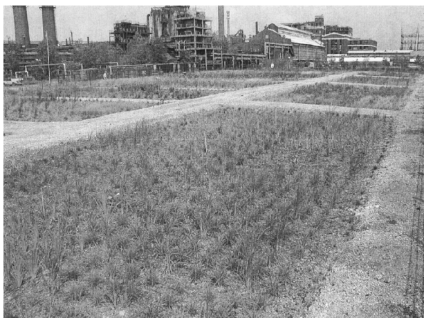
Fig. 1 Experimental phytoremediation installation 1 year after planting at an industrial brownfield site impacted with polyaromatic hydrocarbons (PAHs) (taken August 2003). Approximately 20,000 regional native plants of 22 species are planted in 12 separate plots (each 40 × 90 ft) with distinct plant combinations and habitats (e.g., upland or wetland). The installation covers a 1.6-acre area and will be monitored for 3–5 years for in situ treatment of nearly 4100 cubic yards of contaminated soil in addition to the study of plant community dynamics during the site restoration process.
