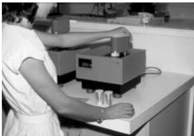
Fig. 7 The Rapid Visco Analyzer, used to determine Stirring Number values. A suspension of milled grain is placed in a disposable cup, clamped in a heating block. The apparent viscosity of the suspension is measured continuously during stirring. A low viscosity after three minutes indicates that the sample is sprouted. (View this art in color at www.dekker.com .)
