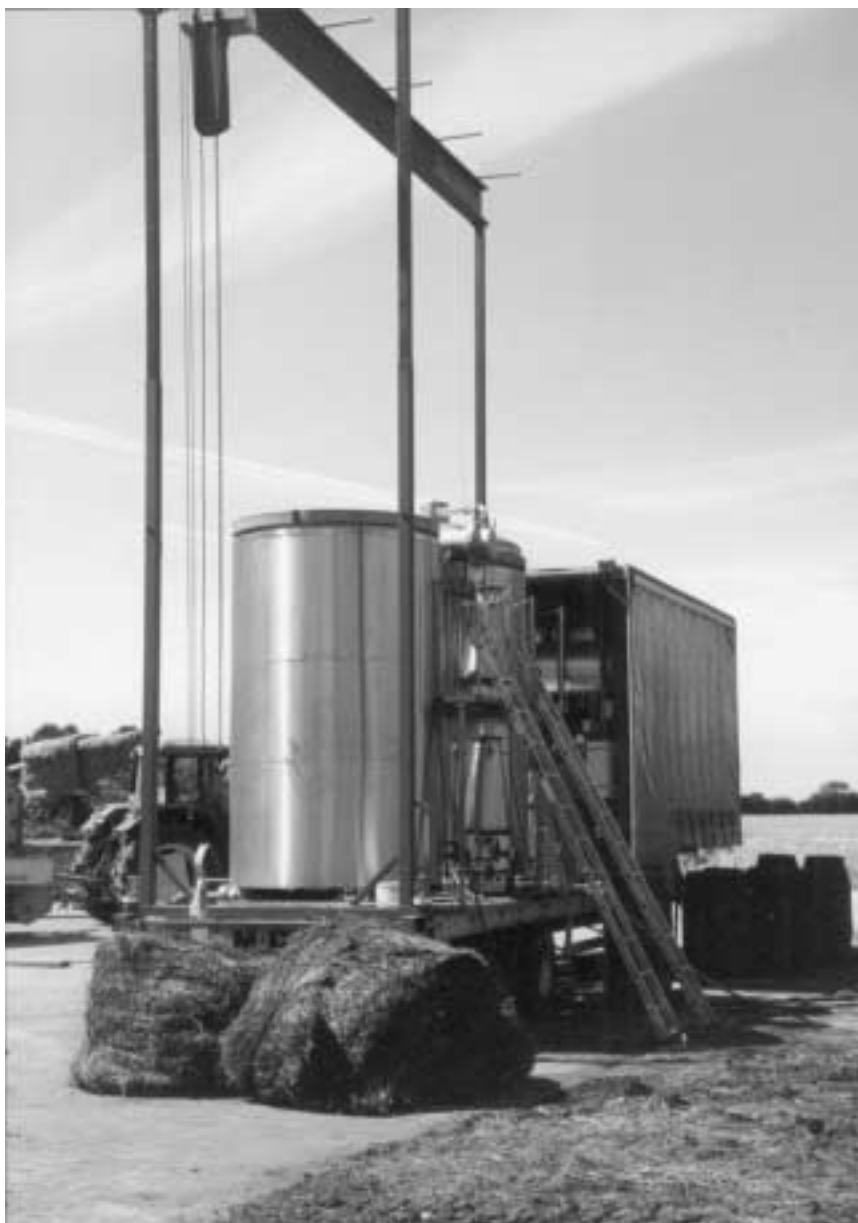
Fig. 2 Field-scale mobile distillation equipment for chamomile harvest. Norfolk, UK, summer 2001. (View this art in color at www.dekker.com .)
