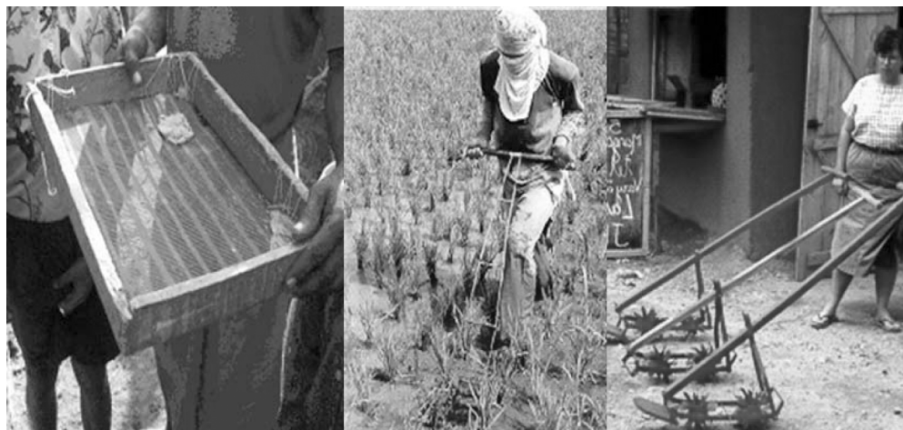
Fig. 2 Sieving and mechanical weeding in developing countries: (A) Sieving out weed seed, (B) Rotary weeder in use, (C) Rotary weeders on display. (View this art in color at www.dekker.com .)
