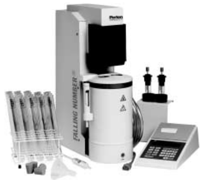
Fig. 6 Falling Number equipment. A suspension of milled grain is mixed with water in a long glass tube immersed in boiling water, using the vertical movement of a plunger. After 60 seconds of mixing, the plunger is raised and allowed to fall under its own weight. Falling time is long for a sound sample but is short if the amylase of sprouted grain has hydrolyzed the starch of the suspended grain particles. (View this art in color at www.dekker.com .)
