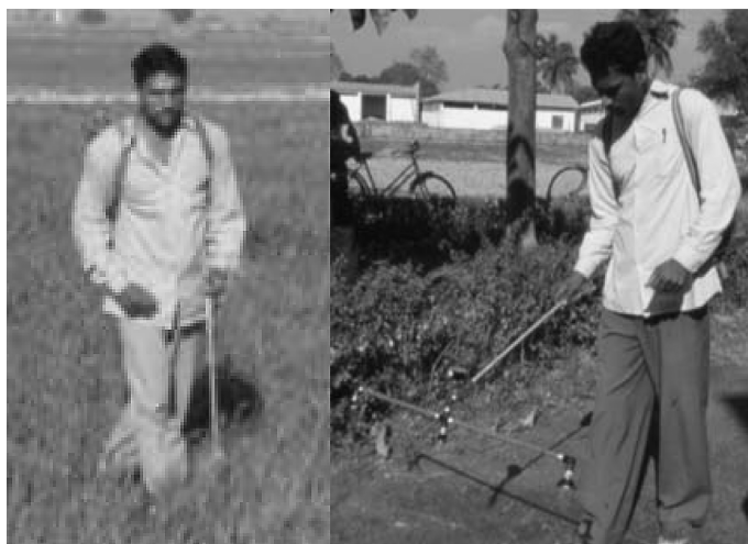
Fig. 3 Traditional (one-nozzle) spray boom (left) and improved (three-nozzle) spray boom (right). (View this art in color at www.dekker.com .)
