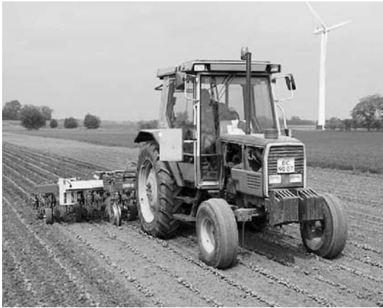
Fig. 1 Automatic steering of an interrow cultivator in radish using a camera (yellow box on the cultivator) for electronic row detection. (View this art in color at www.dekker.com .)
